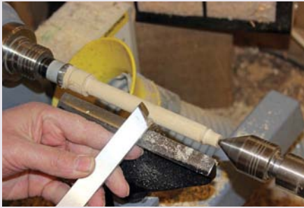
A planing cut using the skew chisel
