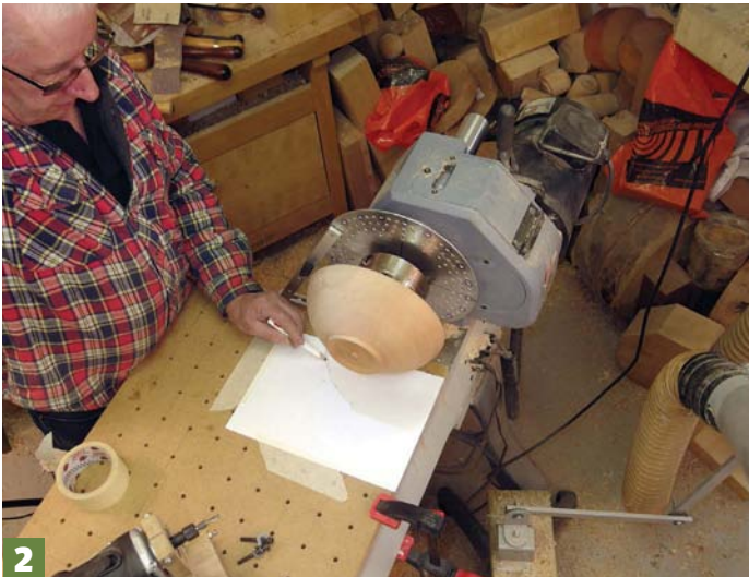
2 Draw around the shadow, cut out the shape and then lay this on top of a suitable piece of thick ply or MDF and cut the shape to match the paper template
