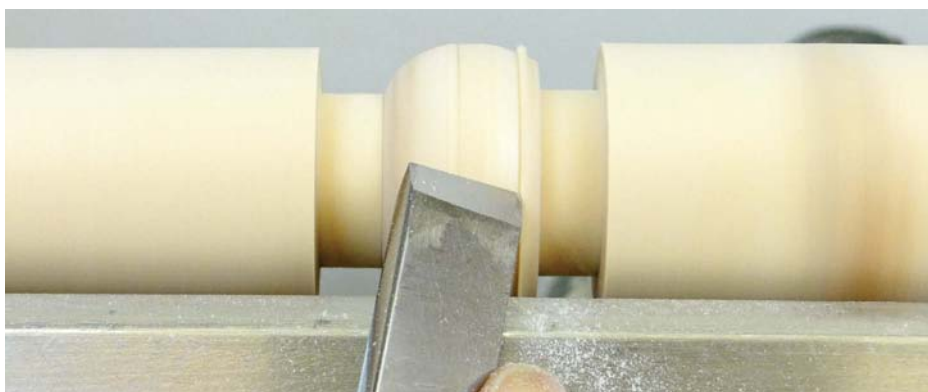
When cutting correctly with the very tip of the tool, the tip sits in a V-groove and a feathered edge is lifted in front of the cut. These are tell-tale signs that you are doing it correctly
