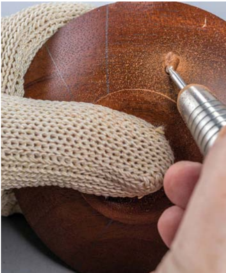
A Kevlar carver's glove can provide protection to your workholding hand when needed. When slips occur, cutters and burs are oblivious to what material they cut
