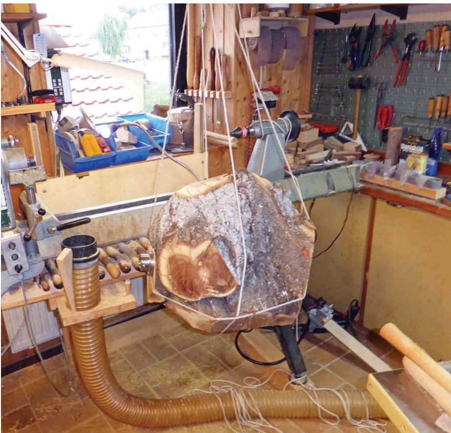
The large burr which the egg was turned from, being hoisted onto the lathe
