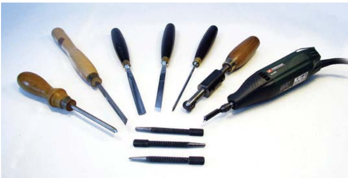
A selection of hand chisels and dedicated turning tools used for texturing
