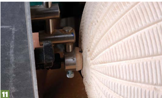
11 Using the router freehand with the shield marked with a blue line so you have a visual reference at which positions to stop the cut
