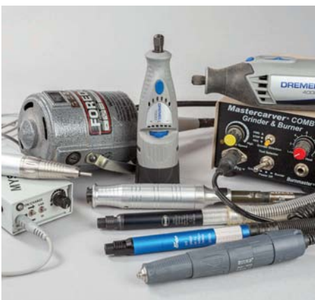
Piercing can be done with one of any of these tools ranging from about £20-265. Your material, thickness and budget will drive your selection
