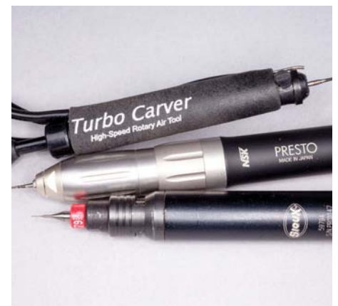
A machine tool grade die grinder and my two favourite high-speed tools. The die grinder is used with thicker materials and the high-speed tools with shell and thin stock
