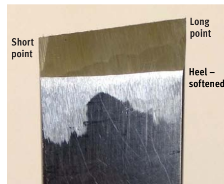
Parts of a skew. Notice my skews are not very skewed in angle compared to some that you might see, which is simply my personal preference
