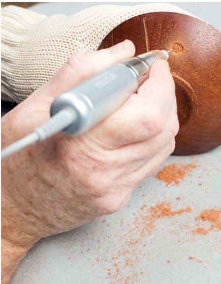
For thicker pieces requiring multiple passes or non-critical depth pockets, the slower speed micromotor tools work well. Depth can be marked on the cutter with tape
