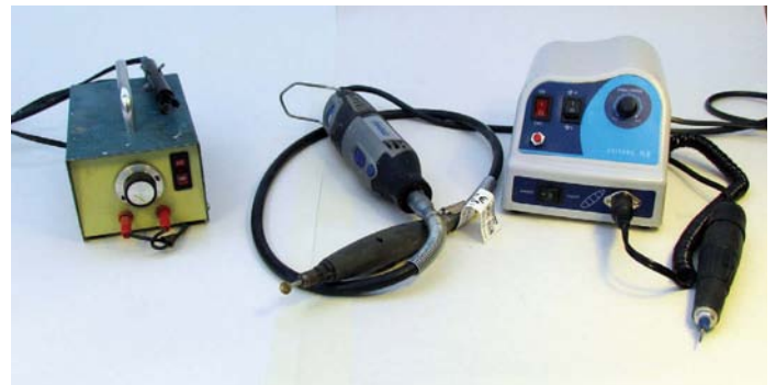
Tools I use including power carvers, a pyrography machine and rotary tools
