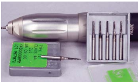
My most used tool and piercing bur design. Notice the manufacturer's speed limit maximum at 450,000rpm. Always heed the cutter and bur speed limitations
