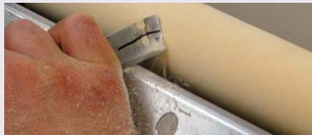
Planing with a skew. Notice the shaving is coming from the 'sweet spot' marked on the edge, giving me a smooth and controlled cut
