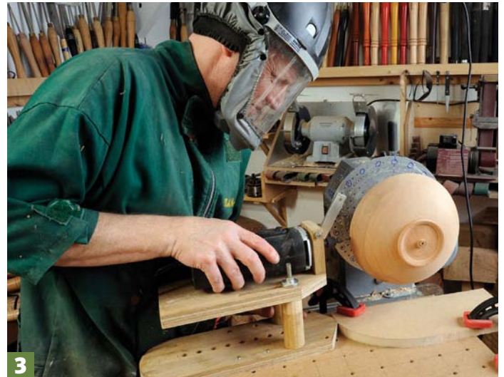
3 Make a follow template or guide to suit the shape being routed
