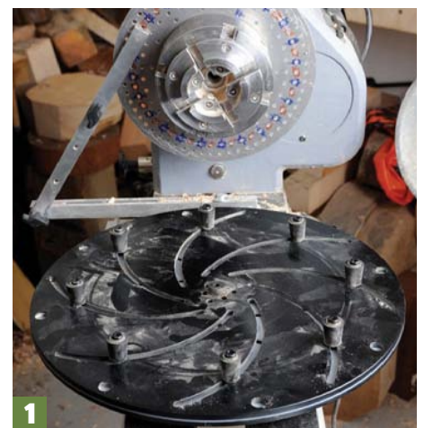
1 Fluting of any sort requires that the work be held in such a way that it is stable while you cut it
