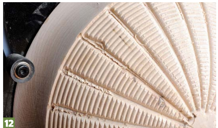
12 One pass with a heavy cut results in the router climbing during the cut, ruining the overall effect. Multiple light cuts are the way to go
