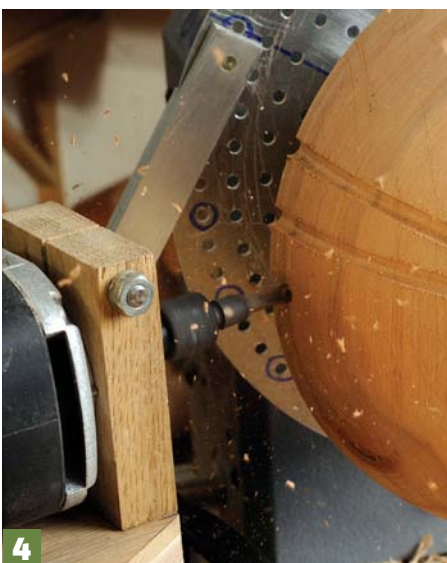
4 Adjust the cutter to give you the required depth. Note the indexing keeps everything in place
