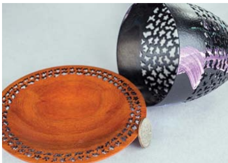
The super high-speed tools lend themselves to shell and thin woods. For best results in wood, a 1-2mm wall thickness works best
