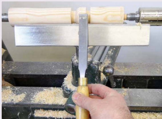
The start and finish positions of the skew when turning the left side of a bead
