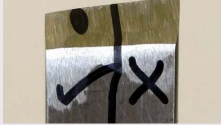
Sweet spot and 'no-go' areas marked on the edge of a skew can be a real help when getting the feel of a skew
